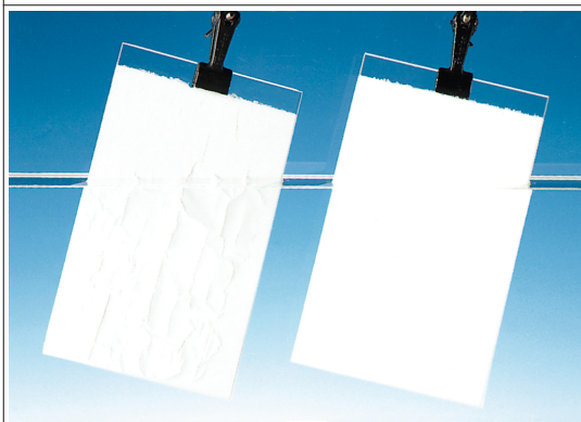
Left glass plate: Conventional emulsion facade paint, right glass plate: Amphibolin.
